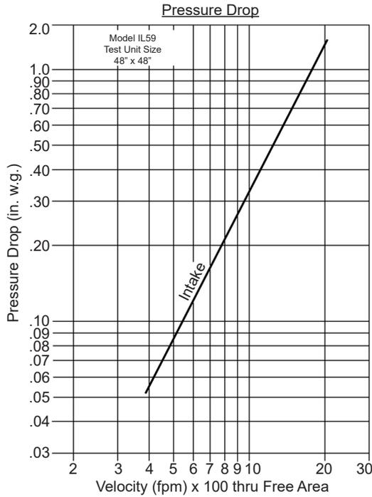
Intake air converted to standard air density.
